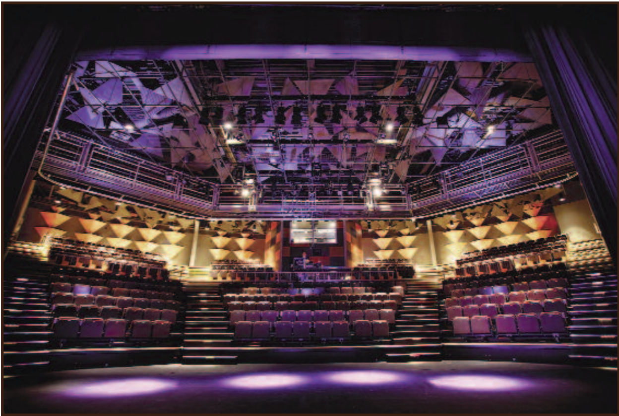
The 174 seats on the lower level are on six rows of Hussey motorized bleachers that, when retracted into the underbalcony cavity, leave a large floor contiguous with the stage area for cabaret-style productions.
