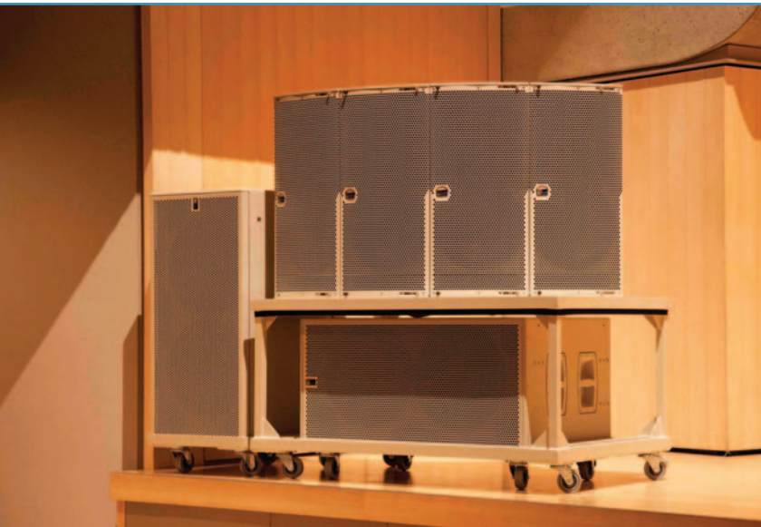
One of the left-right stage-mounted systems comprising four Meyer JM-1Ps and two Meyer 700-HP subs.
